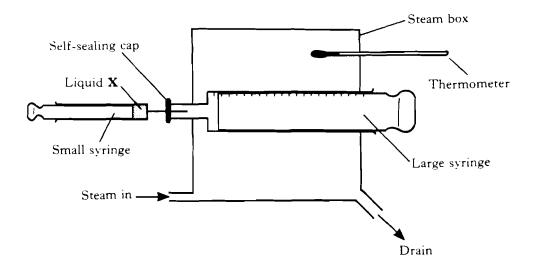
Some of liquid X is injected into the large syringe and it evaporates. The following results were obtained:
